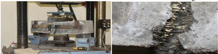
Fig 3.6: Bending test and damaged mode
